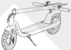
2 Unfold the kickstand (15) on the side of the footrest (10) and place the e-scooter on the floor.
