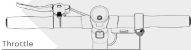
Move the throttle on the right side of the handlebar to start accelerating. You can also accelerate the e-scooter like a conventional push scooter by simply pushing against the floor with your foot.
