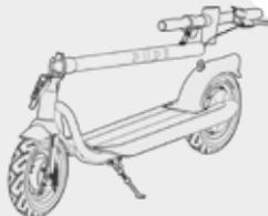
1 Take out the folded e-scooter from the box. Use both hands and lift from the base of the e-scooter. Do not attempt to lift the e-scooter using the stem.
